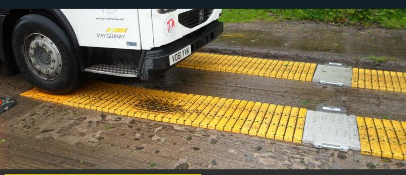
The APOLLO PORTABLE WIM axle weighbridge is a lightweight and robust weighing system, machined from solid aircraft-grade aluminium alloy. It is suitable for weighing vehicles either in-motion (WIM) at speeds of up to 5kmph, or statically, axle by axle. Each pad is rated to 20,000kg, giving a massive capacity of 40,000kg per axle. On a good quality, flat surface, accuracy of +/-0.5% for static weighing and +-2% for low speed weighing-in-motion can be achieved.
