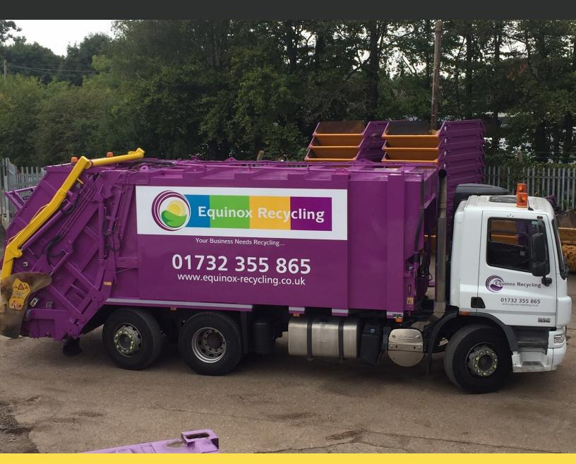
Kent-based Equinox Recycling has noticed a significant impact on its revenue since installing its entire fleet of waste collection vehicles with bin-weighing systems, all of which have been fully weights and measures certified for Pay-by-Weight services. Every collection is weighed to within 1kg and customers are charged according to what they throw.
